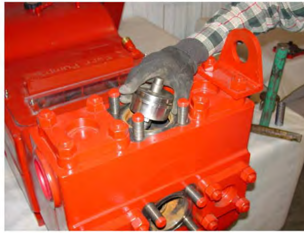
14.) Install the discharge seat and valve. Drive in firmly using bar and hammer.
