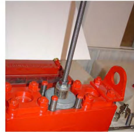
9.) Lifting the puller rod, turn the nut until firmly in contact with the washers.
