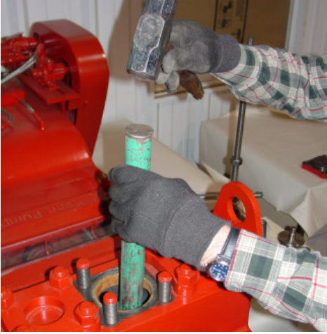
13.) Install the suction seat and valve. Drive in firmly using bar and hammer.
