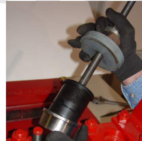
12.) Loosen the puller rod to retract the pins and remove the seat.
