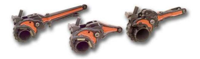
PETOL DRILL PIPE TONGS are designed for making up and breaking out drill pipe, casing, and pneumatic drills on light rigs. These tongs are furnished as original equipment by rig manufacturers because of their ease in handling, quick application, and ability to withstand rugged use.
