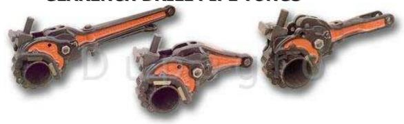
PETOL DRILL PIPE TONGS are designed for making up and breaking out drill pipe, casing, and pneumatic drills on light rigs. These tongs are furnished as original equipment by rig manufacturers because of their ease in handling, quick application, and ability to withstand rugged use.
