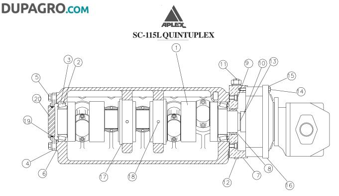
DESCRIPTION: Crankshaft Assy. 2 3/4" Stroke Auburn Planetary Gear #6 R.H. Drive
