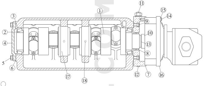
DESCRIPTION: Crankshaft Assy. 2 3/4" Stroke Auburn Planetary #8 R.H. Drive
