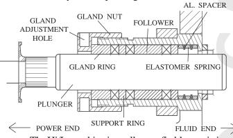
The Hi/Lo packing is totally retrofitable to existing Myers/Aplex pump. Use the drawing for proper reassembly order.
