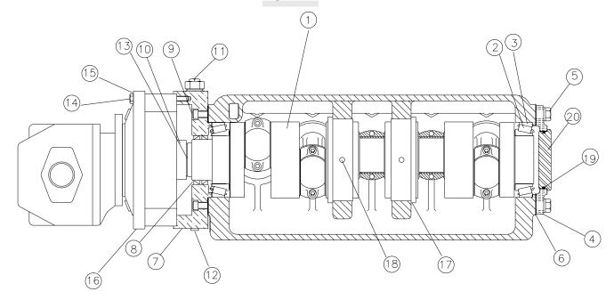
DESCRIPTION: Crankshaft Assy. 2 3/4" Stroke Auburn #6 Planetary Gear L.H. Drive
