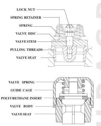
The Myers/Aplex valve is a precision made subassembly utilizing threads cut into the rim of seat for use with Myers/Aplex setting/pulling tool. These threads do **NOT** deteriorate as proven by field experience. By locating these on the rim setting/ pulling forces are now applied only to the rim of the seat, never to the webs (or "spokes"), or to the center section. Distortion of the seat is eliminated.
