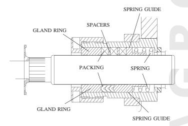
Note that the gland is screwed tightly onto the box and contacts its face. The spring is providing all of the initial compression and adjustment. No adjustment is provided by the gland.
