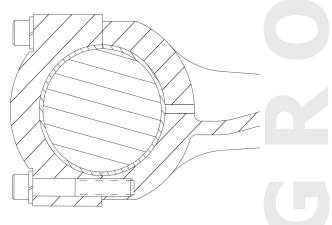
Check that all oil holes are clean and fully open. **GRIT** is the greatest enemy of bearings, however precisely manufactured. Hence, all surfaces must be perfectly clean and lightly oiled prior to assembly. Remove any burrs or sharp corners which prevent the perfect fitting of these precision bearings. Using a torque wrench, tighten cap bolts as follows:
