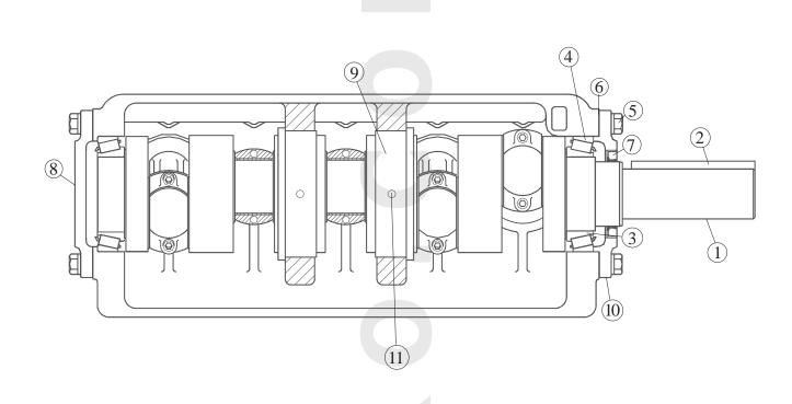
DESCRIPTION: Crankshaft Assy. 2 3/4" Stroke Right Hand and Left Hand Drive Right Hand Shown
