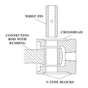
A mishap during insertion can occur causing the ruin of the pin or the crosshead, *if* during application of pressure:
