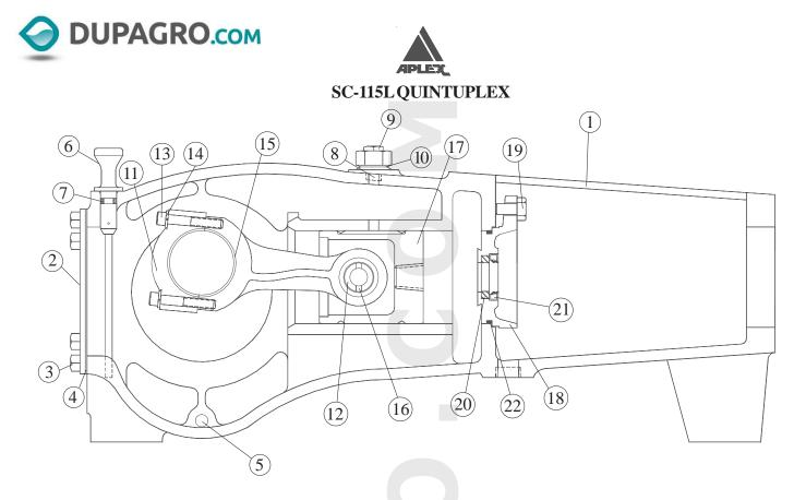
DESCRIPTION: Power Frame Assembly; Conn. Rod, Crosshead & Wiper Box Assembly
