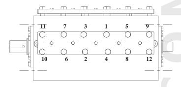
Failure to fully and *evenly* tighten these studs (or cap screws) can lead to early failure, plunger misalignment and failure, and short packing life. Retighten after 500 hours of operation.
