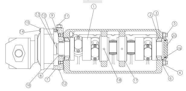
DESCRIPTION: Crankshaft Assy. 2 3/4" Stroke Auburn Planetary #8 L.H. Drive
