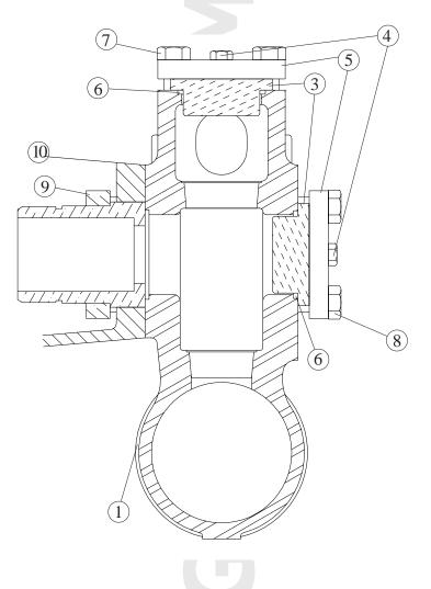
DESCRIPTION: Side Suction Fluid End Assembly, Ductile Iron
