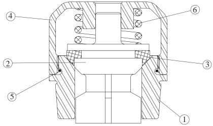
DESCRIPTION: Abrasion Resistant Valve Assembly Parts Assembly TS20-AR0-AC0716 Suction Need 5 per pump
