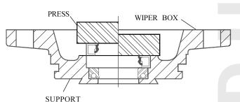
The mechanical seal contains a garter spring. Check to see that this spring is still properly located and in its position. The mechanical seal has a metal case which serves to force the "Poly Pak" seal into its cavity, energizing its lips. Apply oil lightly to the bore of the box before pressing each seal into its counterbore.
