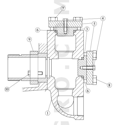
DESCRIPTION: Fluid End Assembly, Ductile Iron
