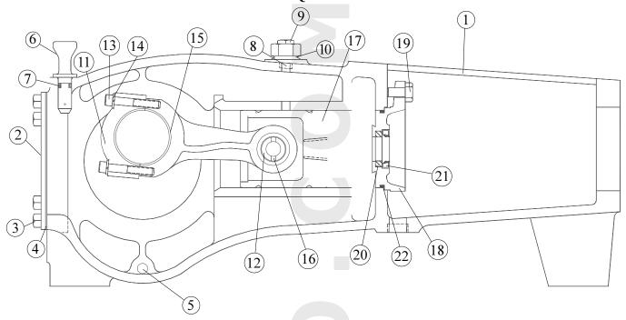
DESCRIPTION: Power Frame Assembly; Conn. Rod, Crosshead & Wiper Box Assembly PE185 and Five PE137
