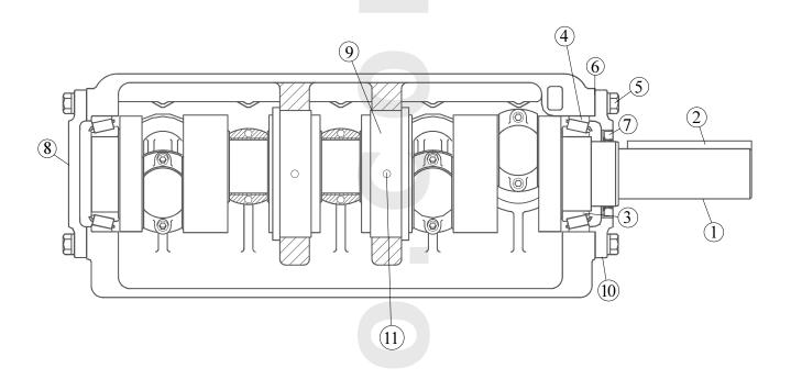
PE155 DESCRIPTION: Crankshaft Assy. 2 3/4" Stroke Right Hand and Left Hand Drive Right Hand Shown
