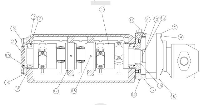
PE291 DESCRIPTION: Crankshaft Assy. 2 3/4" Stroke Auburn Planetary Gear #6 R.H. Drive
