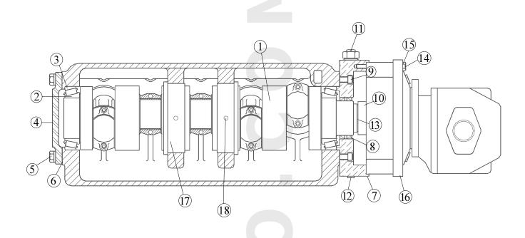
PE221 DESCRIPTION: Crankshaft Assy. 2 3/4" Stroke Auburn Planetary #8 R.H. Drive
