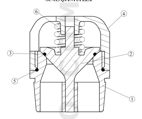
DESCRIPTION: Dual Stem Guided Valve Assembly Available Assembly TS18-SG0-AC0478 Need 10 per pump
