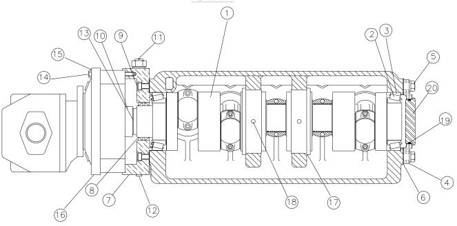
PE266 DESCRIPTION: Crankshaft Assy. 2 3/4" Stroke Auburn #6 Planetary Gear L.H. Drive
