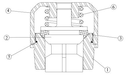
DESCRIPTION: Abrasion Resistant Valve Assembly Parts Assembly TS18-AR0-AC0714 Suction
