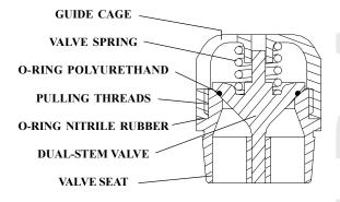
The Myers/Aplex valve is a precision made subassembly utilizing threads cut into the rim of seat for use with Myers/Aplex setting/pulling tool. These threads do **NOT** deteriorate as proven by field experience. By locating these on the rim setting/pulling forces are now applied only to the rim of the seat, never to the webs (or "spokes"), or to the center section. Distortion of the seat is eliminated.
