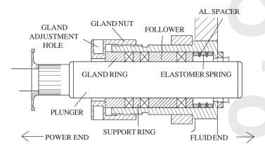
The Hi/Lo packing is totally retrofitable to existing Myers/Aplex pump. Use the drawing for proper reassembly order.
