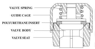
The Myers/Aplex valve is a precision made subassembly utilizing threads cut into the rim of seat for use with Myers/Aplex setting/pulling tool. These threads do **NOT** deteriorate as proven by field experience. By locating these on the rim setting/pulling forces are now applied only to the rim of the seat, never to the webs (or "spokes"), or to the center section. Distortion of the seat is eliminated.
