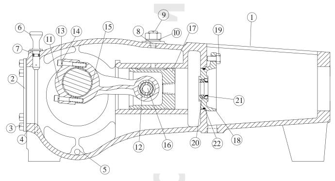
DESCRIPTION: Power Frame Assembly; Conn. Rod, Crosshead & Wiper Box Assembly
