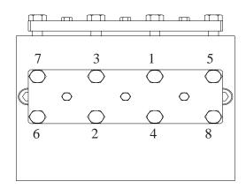
Failure to fully and *evenly* tighten these studs (or cap screws) can lead to early failure, plunger mis-alignment and failure, and short packing life. Retighten after 500 hours of operation.
