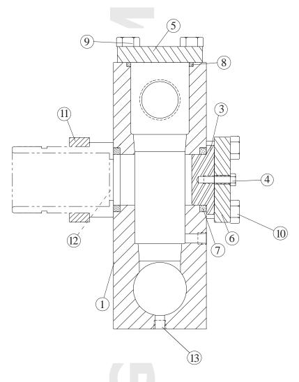
DESCRIPTION: Fluid End Assembly, Carbon Steel
