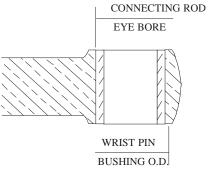
Carefully align the bushing with its hole and after applying oil to bushing O.D. use a hydraulic press to force it home. When a bronze bushing is pressed into
