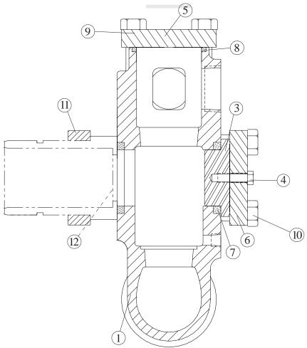
DESCRIPTION: Fluid End Assembly, Ductile Iron
