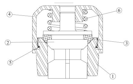
DESCRIPTION: Abrasion Resistant Valve Assembly Parts Assembly TS18-AR0-AC0714 Suction Need 3 per pump
