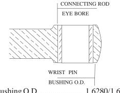
Carefully align the bushing with its hole and after applying oil to bushing O.D. use a hydraulic press to force it home. When a bronze bushing is pressed into
