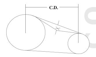
Sheaves must be balanced to prevent abnormal vibration. Balancing weights must **NOT** be removed. Type "QD" sheaves must be evenly tightened on their tapered hubs to avoid rim wobble and severe lateral vibration. V-belts which snap and jerk will produce abnormal vibration and loads on both pump and motor or engine.
