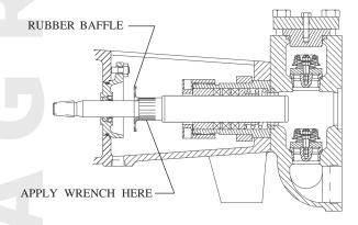
Fasten the wiper box to the power frame by evenly tightening the two nuts on the wiper box studs. Oil leakage between frame face and wiper box is prevented by an o-ring on the O.D. of the wiper box.
