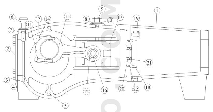
DESCRIPTION: Power Frame Assembly; Conn. Rod, Crosshead & Wiper Box Assembly
