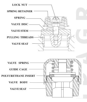
The Myers/Aplex valve is a precision made subassembly utilizing threads cut into the rim of seat for use with Myers/Aplex setting/pulling tool. These threads do **NOT** deteriorate as proven by field experience. By locating these on the rim setting/pulling forces are now applied only to the rim of the seat, never to the webs (or "spokes"), or to the center section. Distortion of the seat is eliminated.
