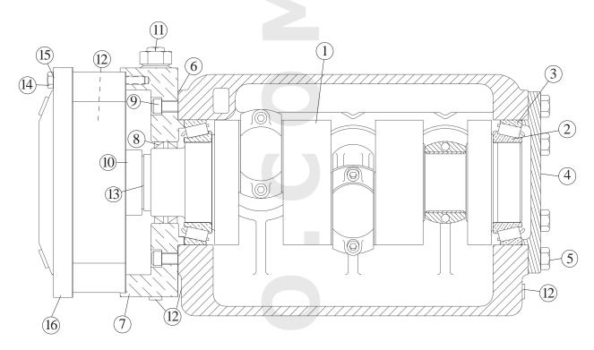
DESCRIPTION: Crankshaft Assy. 2 3/4" Stroke Auburn Planetary L.H. Drive
