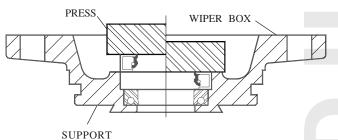
The mechanical seal contains a garter spring. Check to see that this spring is still properly located and in its position. The mechanical seal has a metal case which serves to force the "Poly Pak" seal into its cavity, energizing its lips. Apply oil lightly to the bore of the box before pressing each seal into its counterbore.
