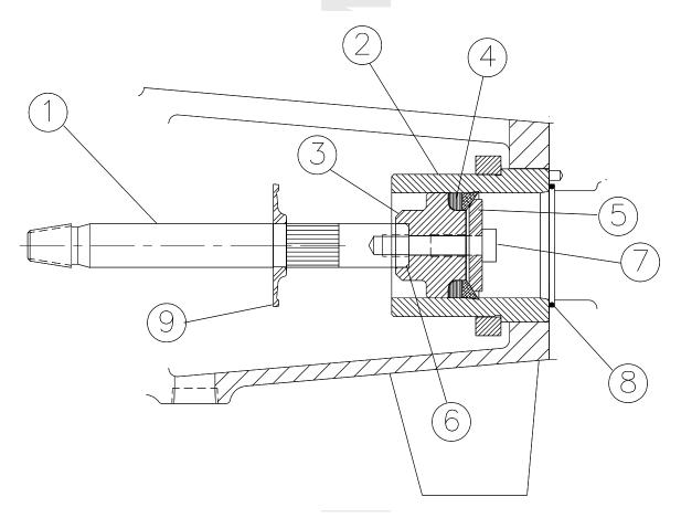
DESCRIPTION: Piston Assembly 3" Black Rubber and White Ceramic Need Three per Pump
