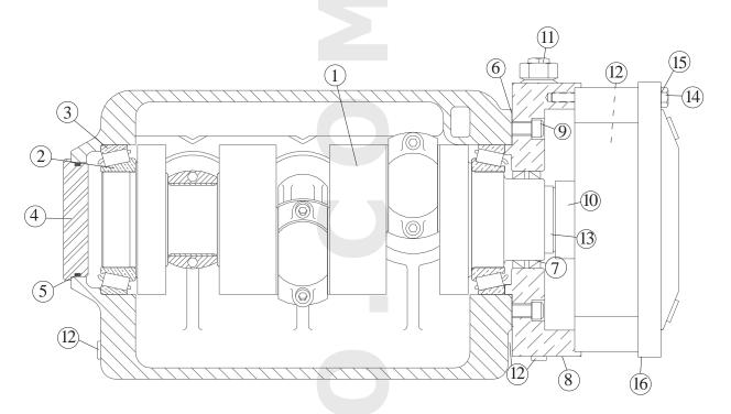
DESCRIPTION: Crankshaft Assy. 2 3/4" Stroke Auburn Planetary R.H. Drive
