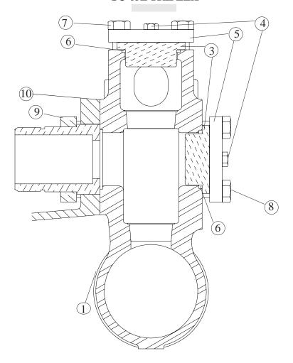
DESCRIPTION: Side Suction Fluid End Assembly, Ductile Iron
