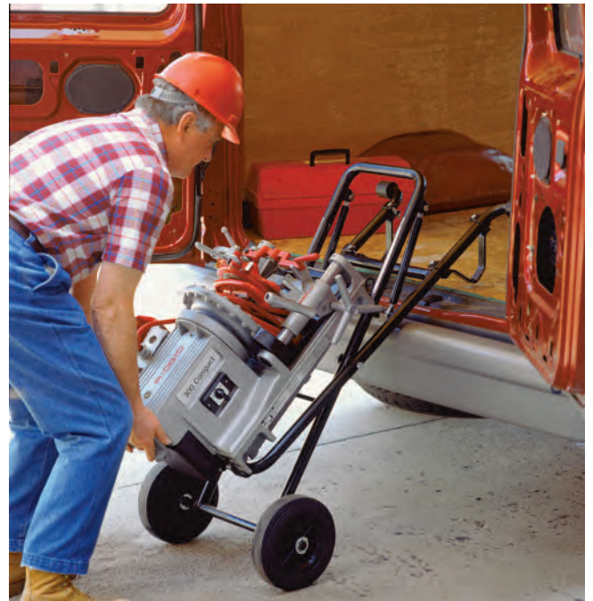
Model 300 Compact is a versatile choice for threading and roll grooving applications.
