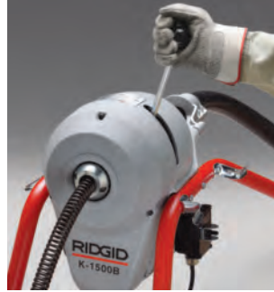
Release handle, cable stops instantly
