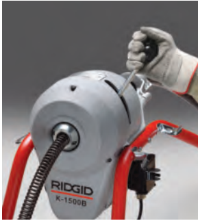
Engage clutch, cable spins
