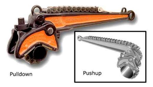
PETOL VISETONGS are designed to operate best when large makeup torques are required and when heavy loads are needed to breakout tool joints, drill collars, reamers, and similar heavy jobs. A hydraulic cylinder can be attached to the end of the tong handle.
